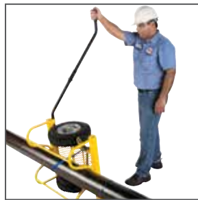
2 Use handle to flip Cricket & pipe
