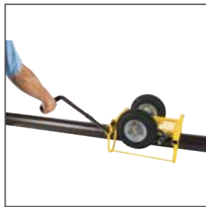
1 Use ratchet to secure Cricket to pipe
