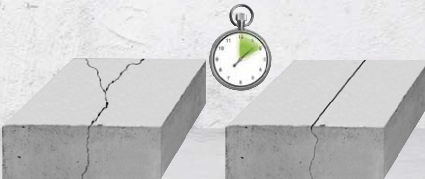
Random cracking in concrete
