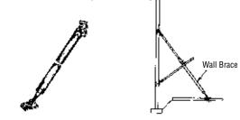
**Brace Inserts** are available in several versions. They are designed to be cast-in-place and used to anchor tilt-up wall braces during the construction sequence.
