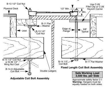
**Type 7** is similar to the standard Type 1 hanger but has the capacity to accommodate haunch heights up to 1-1/2".
