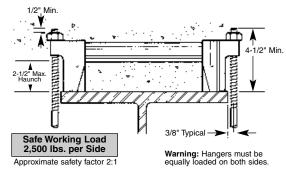
**Type 4** is fabricated with two 90° 1/2" interlock type end sections welded to a substantial wire strut. It is a high strength hanger used to support bridge deck interior formwork and is especially designed to react to lateral forces prevalent in many forming conditions.
