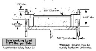
**Type 8** is similar to the standard Type 1 hanger except the two 1/2" end sections are set at 15° to provide additional clearance for supporting the deck formwork.
