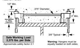
**Type 3** is similar to the Type 2 hanger but is manufactured with a corrugated connecting strap instead of a wire strut. The Type 3 hanger provides up to a 2-1/2" maximum haunch height.
