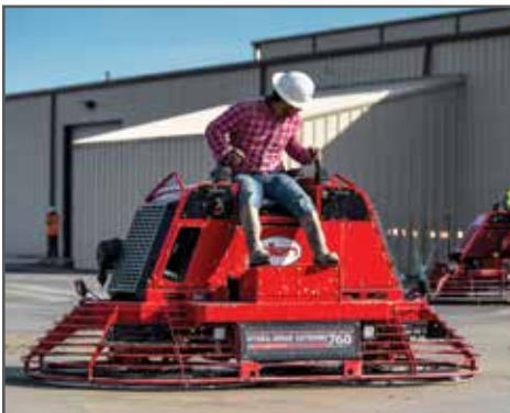
The powerful 74 hp Hatz Tier IV Final engine will provide all the power you will need for any job size.
