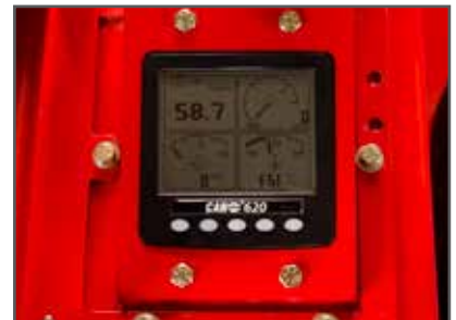
The digital display will allow you to see rpm, temperature, hours, and more in one convenient place.
