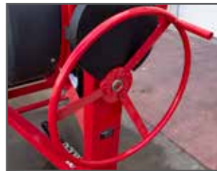
Oversized drum wheel makes discharge of material easier.
