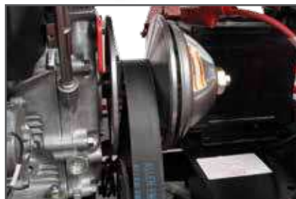
The torque converter clutch ensures maximum control over machine speed.
