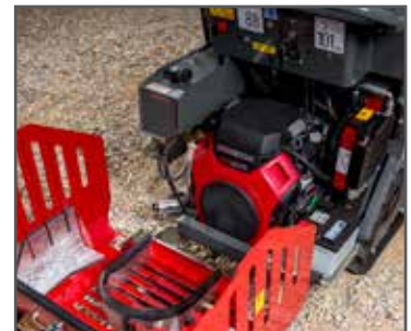
Engine cover folds back to provide convenient access to the engine, gasoline tank, battery, and filters.
