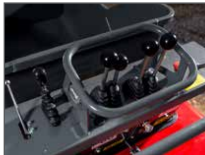
Two servo levers control the direction of the machine, and they automatically reset to stop in case of emergency.
