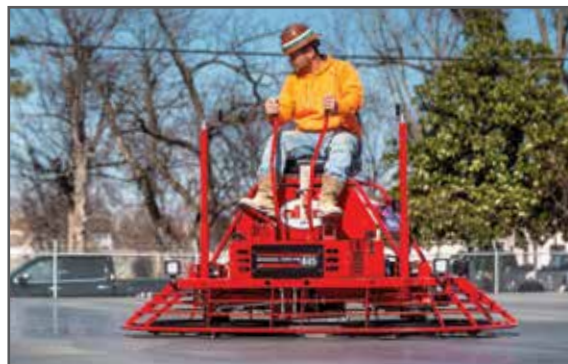
The torque converter clutch ensures maximum control over machine speed.
