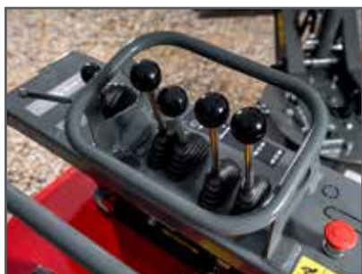
Two servo levers control the direction of the machine, and they automatically reset to stop in case of emergency.
