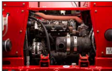
The powerful 74 hp Hatz Tier IV Final engine will provide all the power you will need for any job size.
