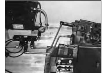
Simplex spring return cylinders, used in this fabricating fixture, provide fast and accurate forming of precision metal products.
