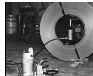
Large steel coils that were damaged in handling are reshaped using a Simplex R256 cylinder and 70 Series pump.
