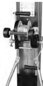
Sumner-built Winch – Highly reliable, single-speed winch uses idler roller to feed four rollers to feed cable evenly on the drum to avoid cable flats.
