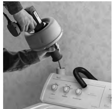
The 3/8" cable in the K-39-5 and K-39-7 extends machine's capacity to 2½" drain lines.
