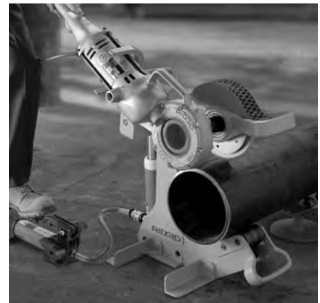
Model 258 Pipe Cutter with No. 700 Power Drive in use for cutting.
