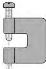
C-CLAMP WITH LOCKING NUT
