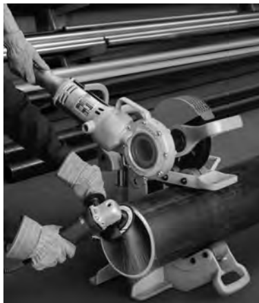
Model 258 with Pipe Roller in use for beveling. Two operators are recommended for this operation.
