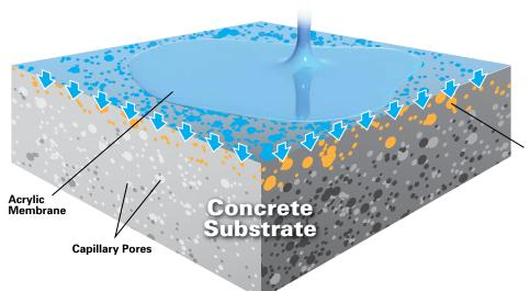
ChemMasters 1 Step Cure & Seals contain an integral silane sealer that penetrates deeply into concrete pores and capillaries where it reacts to form a water repellent silicone for long-term protection against damage caused by freeze/thaw cycles and deicing chemicals. Cure your concrete and add a Silane Shield for enhanced durability, all in one application.
