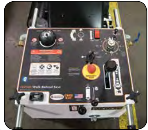
CC2500 control panel shown with optional raise/lower control switch
