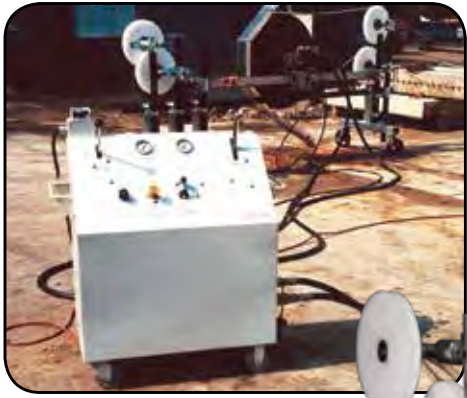
Wire Saw Control Station
