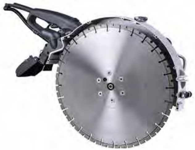
Removable guard side for flush cutting (Flush-cut bolt pattern required on blade in order to cut flush)
