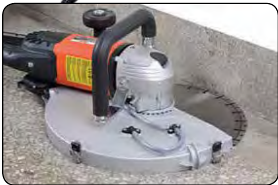
Flush cutting is easy with removable side guard
