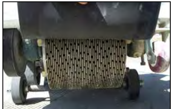
Uses 12" (30.48cm) diameter blades on a 10" (25.4cm) or 16" (40.64cm) grinding head with specifications that can be custom fit to your application
