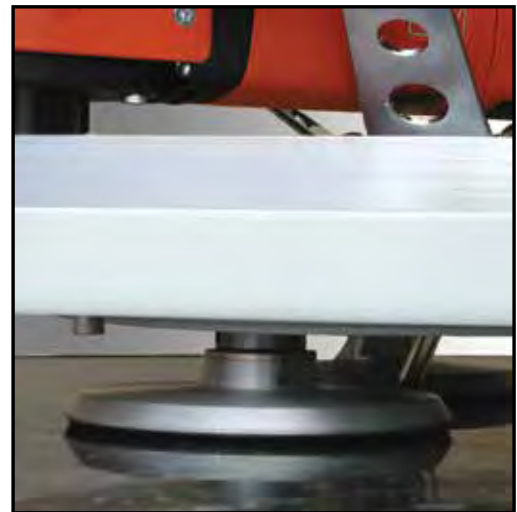
One of three 5" grinding platens (Velcro® surface)
