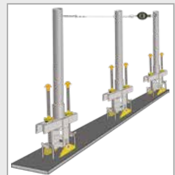
Intermediate Span Installation
