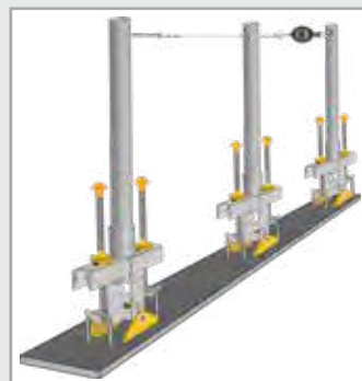
Intermediate Span Installation
